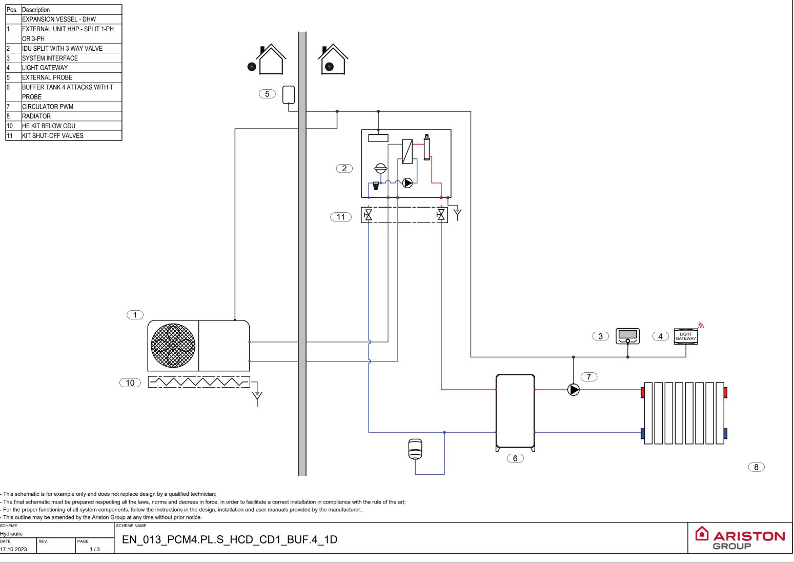
This schematic is for example only and does not replace design by a qualified technician;
