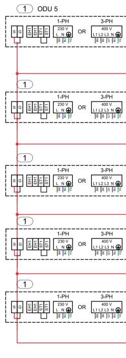
ATTENTION: The power supplies of each indoor and outdoor unit must be connected separately to dedicated residual-current circuit breakers as indicated in the installer manuals
