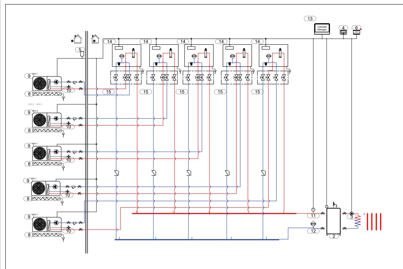
(\*) To be opened in case of DHW enabled for the related HHP
