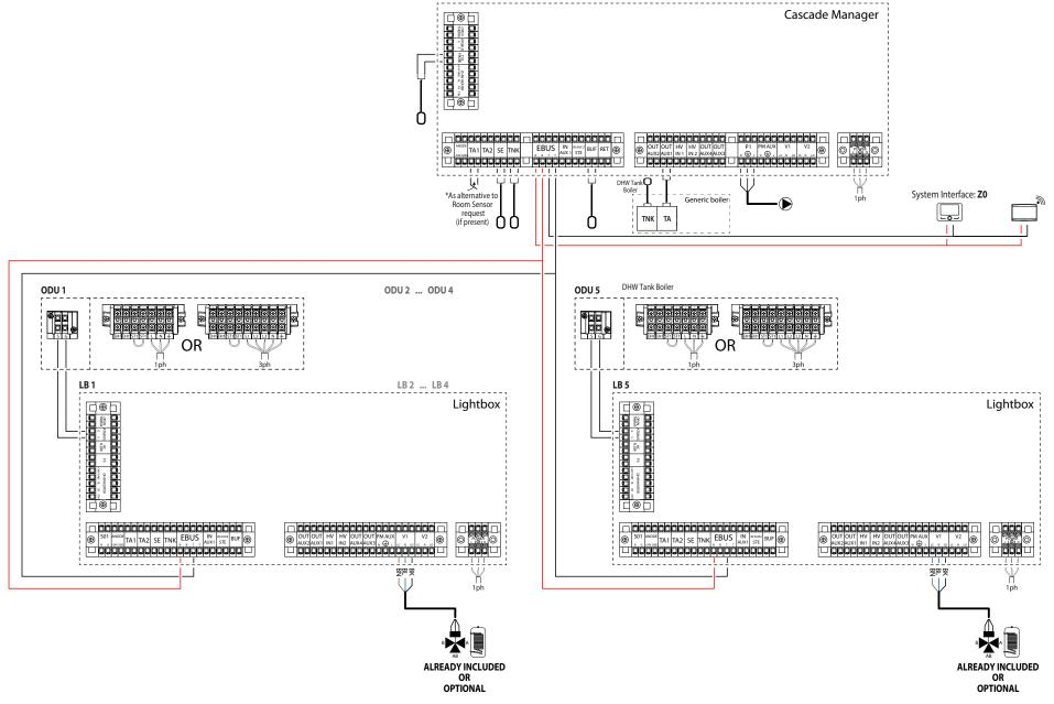
The power supplies of each indoor and outdoor unit must be connected separately to dedicated residual-current circuit breakers as indicated in the installer manuals
